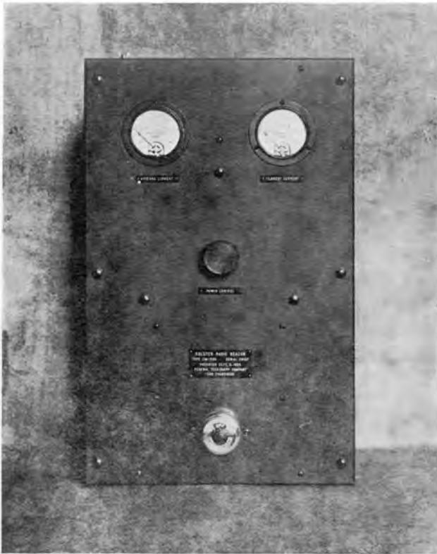
Radio Beacon Type CM-1530, developed by Frederick A. Kolster. It was manufactured by the Federal Telegraph Company in 1927.
